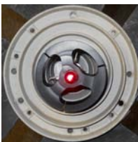
PHOTO A Focal Finder to Locate Center of Antenna
